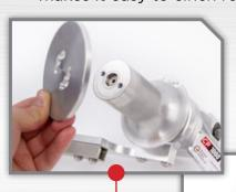
line to start a pull. Lines slip off easily from capstan at completion. The new capstan end plate attaches to the capstan for greater line capacity.
